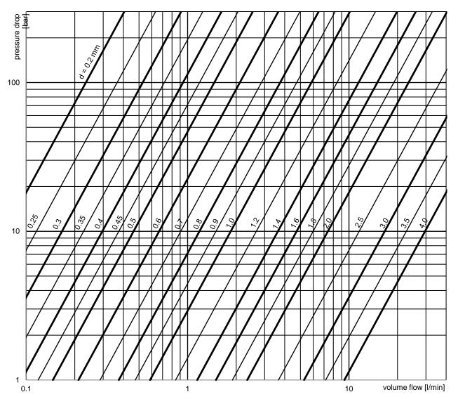
Flow coefficient approx. 0.5 Density 0.9 kg/dm<sup>3</sup>
