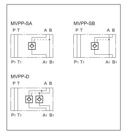
MVPP PILOT OPERATED CHECK VALVE SERIES 50
