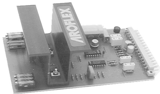
The current stabilising control card EA, controls the DC-solenoids of analogue valves (proportional valves) supplying a constant current, independent of coil temperature and resistance.
