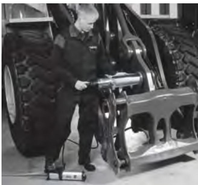
PP70-1000 pump, equipped with AMT801 pressure gauge and AVM204 pressure gauge adapter to display hydraulic pressure.
