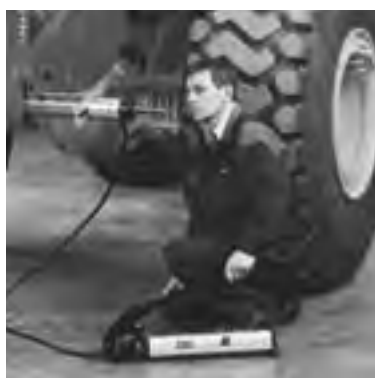
Replacement of a bushing using a hollow cylinder and hand pump.
