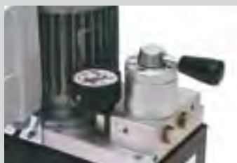
All electric pumps can be fitted with an AMT801 pressure gauge with the aid of the AAM14 pressure gauge adapter.
