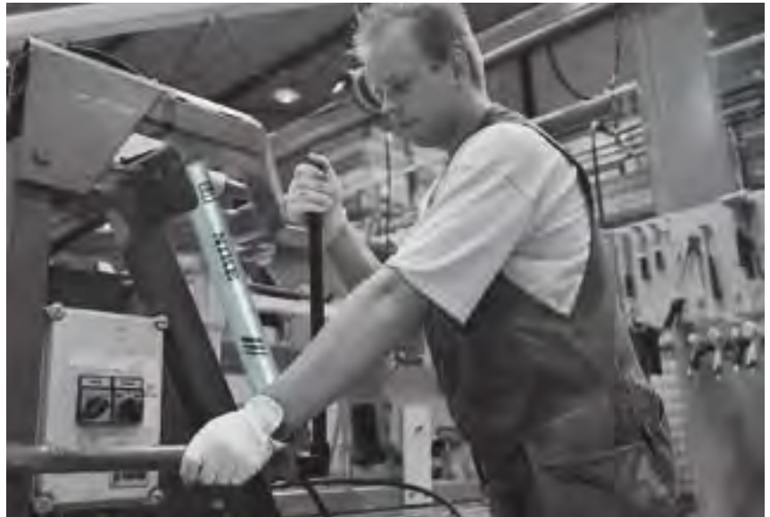
NIKE hand pump used as a power source in an assembly jig for fitting parts to an industrial robot.
